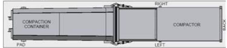
Typical Installation Layout
